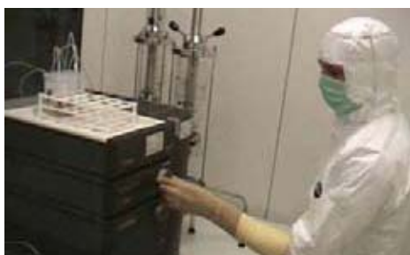
Fig 8 (Above and below) AKTA Explorer 100air connected to BPG column; KTA system in operational.
